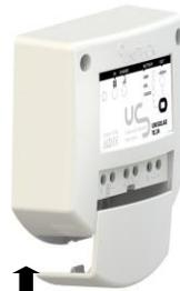
❷ Close the cover by pushing from the bottom to the top
